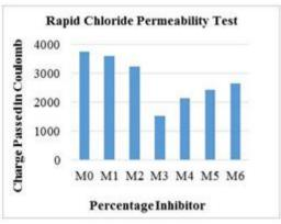
Fig 6: Rapid chloride permeability test
