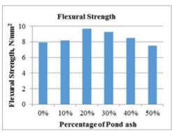
Fig 5: Flexural strength
