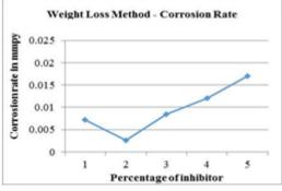
Fig 7: Corrosion rate-weight loss method
