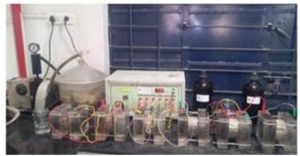
Fig 1: Rapid chloride permeability test
